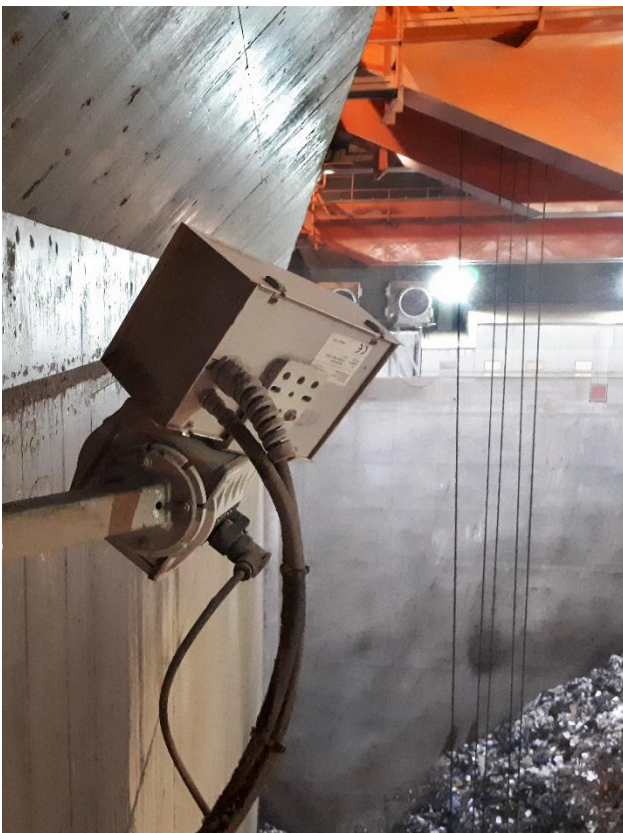
Fig. 2: The camera heads designed as twin systems are integrated in special protective housings which offer protection against dirt, dust, moisture and heat. Together with the pan-tilt systems, they form an effective unit in 24/7 operation.
